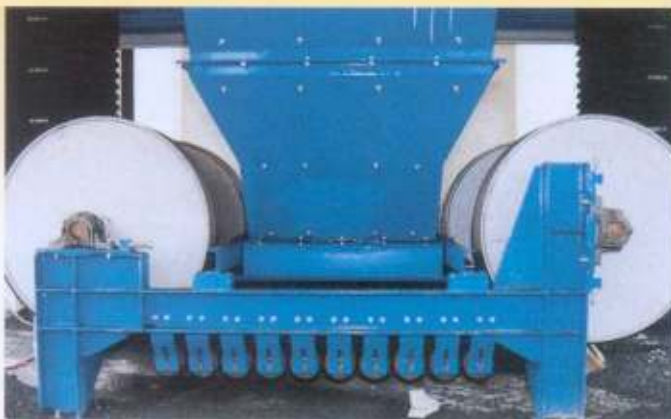
Inner conveyor, bottom station ferro-alloy, 250 t/h
