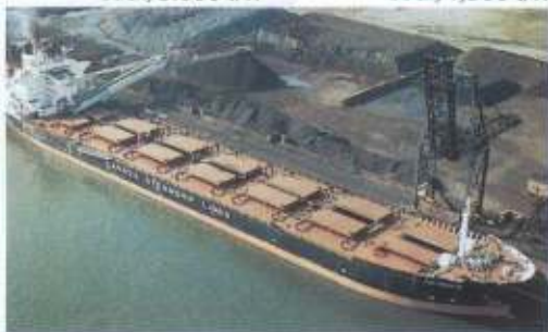
Self unloading vessel, iron ore, 5,000 t/h
