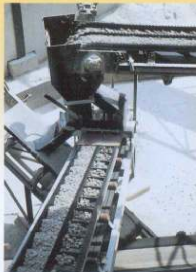
FLEXOWELL®-conveyor belts with centre profile, 2 gravel sizes, each 80 t/h
