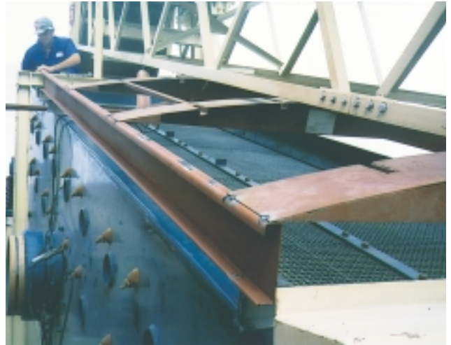
Top frame on RHS profiles
